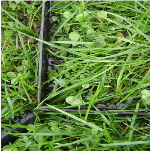
Photo 3. Part of a collection frame with overland flow visible.
