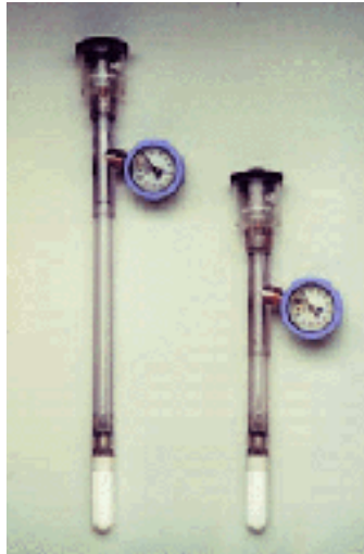
Fig. 2. Tensiometers showing pressure gauge and ceramic cup at the base
