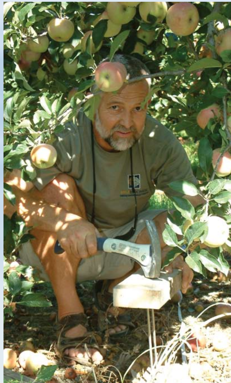
Figures 5: Dan Bloomer installing the TDR rods to measure soil moisture content.
