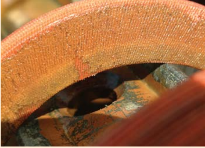
Picture 2. Close up of filter rings, cleaning desperately needed.
