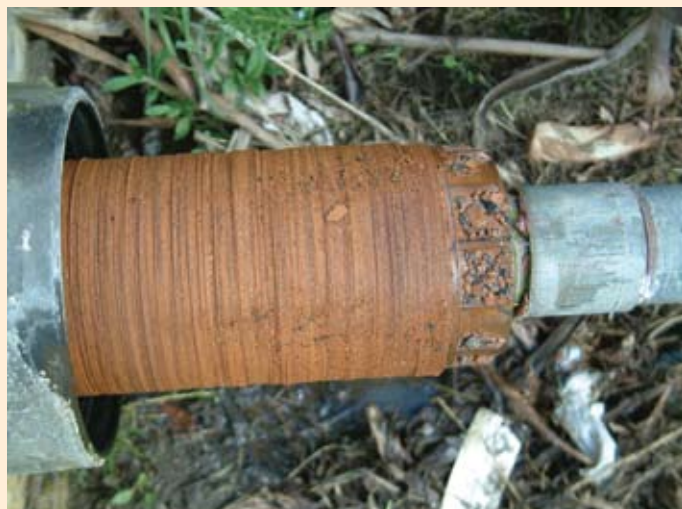
Picture 1. Inside a filter clogged with sand and iron. Cleaning this blocked ring filter slashed pressure losses, increasing irrigation performance and reducing energy consumption.
