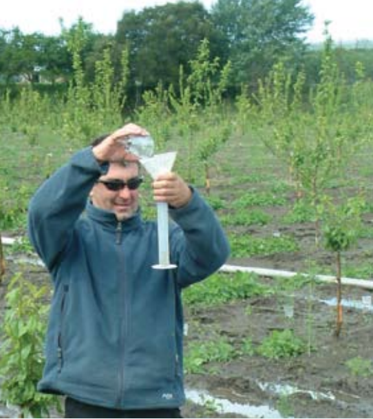
Figure 3: Measuring water collected in disposable wineglass, collectors in grid visible in background.
