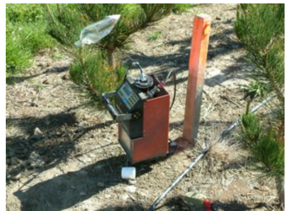
A neutron probe measuring soil moisture in a Radiata pine breeding nursery
