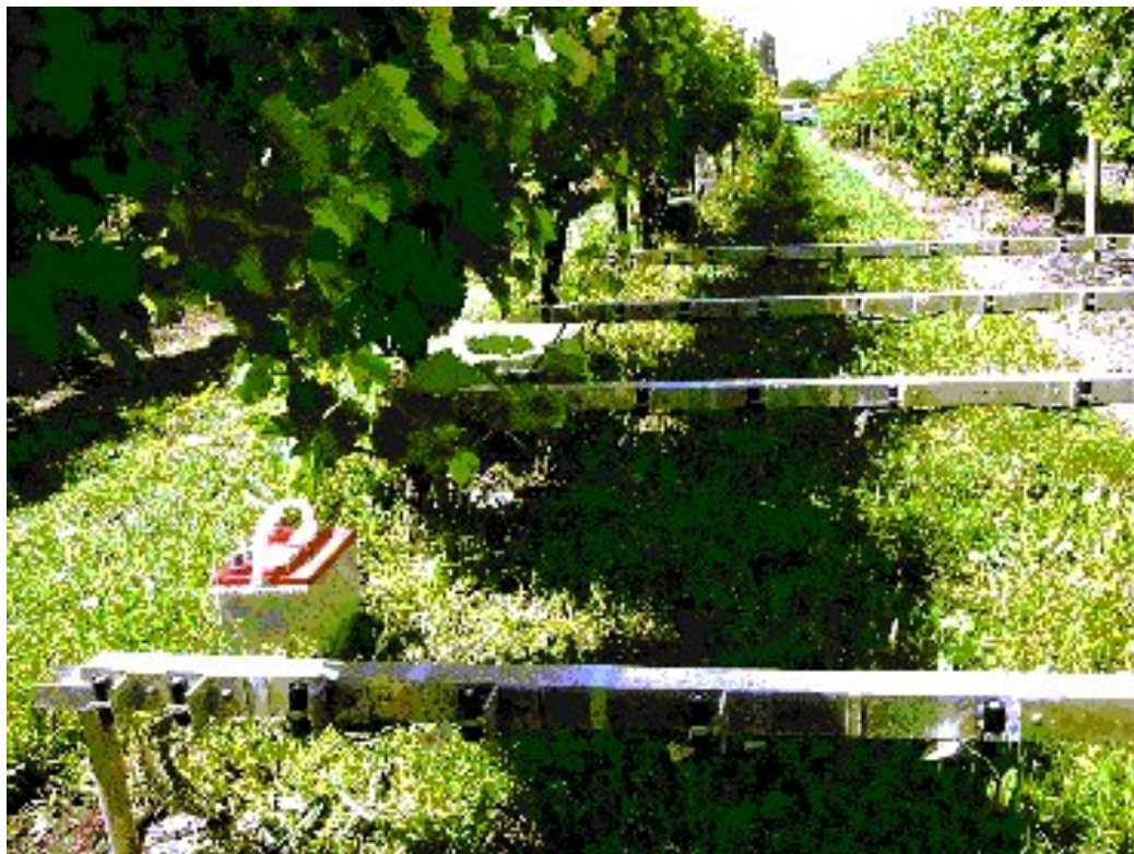
Figure Four Light sensors for measuring light interception.
